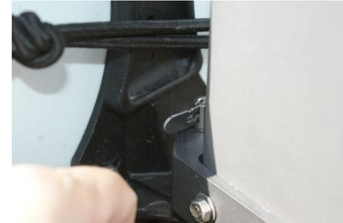
The Jib is a simple.. pull on the blue rope on the side of the mast. Pull from below the pulley and cleat off. Needs quite a bit of force to get it tight. Leave forestay attached.
