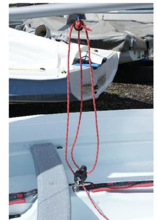
Putting the H12/2 away. Simply reverse the process from putting everything up! Attach the cover using the main halyard to raise the cover so it does not pond.
