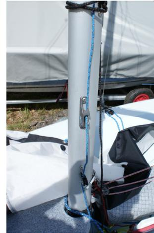
To hoist the main sail make sure the main halyard is through the eye in the top of the sail, and pull the red halyard on the other side of the mast. And cleat off.
